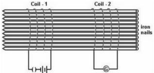
Two coils of insulated copper wire are wrapped on few long iron rods. Coil-1 is connected to a battery through a switch and Coil-2 is connected to a galvanometer. Now, the current is switched on in Coil-1. A momentary deflection is seen in the galvanometer attached to Coil-2. The deflection is due to current induced in Coil-2 momentarily as the magnetic field builds up along the axis of Coil-1 when the current is switched on.
